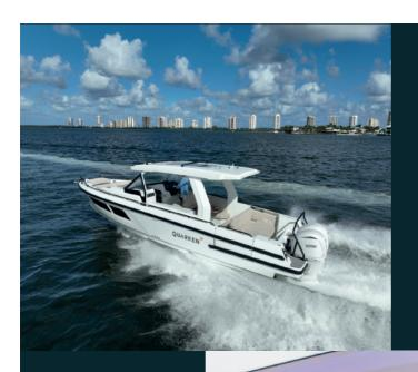
The Quarken 35 ST is designed, produced and assembled in Finland. The hull is manufactured by vacuum infusion technology that offers benefits as thickness control of the GRP and quality consistency in the production process. The outcome is a strong, nimble and lighter hull with lower fuel consumption. <
