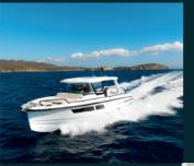
The Quarken 35 GT is designed, produced and assembled in Finland. The hull is manufactured by vacuum infusion technology that offers benefits as thickness control of the GRP and quality consistency in the production process. The outcome is a strong, nimble and lighter hull with lower fuel consumption.
