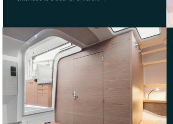
An enclosed toilet compartment that seamlessly follows the same style as the rest of the interior in the forward cabin. The head consists of a toilet, sink, shower unit and a mirror that is installed on the door.
