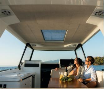
The cockpit area is covered by a solid T-top roof constructure that offers weather protection. The roof includes a glass sky window that provides a light-flooded atmosphere in the cockpit.
