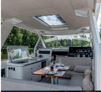
The double helm seat/sofa with height adjusting possibility have a backrest that can be flipped towards the dining area to form an L-sofa in the cockpit. By flipping the backrest of the large aft sunbed to the rear a U-formed dinning area is formed in a blink of an eye.  $\leftarrow$
