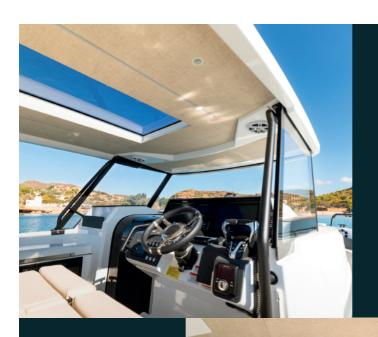
The negative window reduces reflections, improves visibility in bad weather and offers protection together with the robust roof construction.
