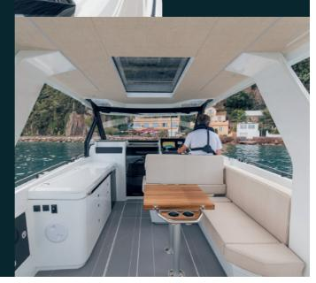
The dashboard and console panels have a high-gloss black finish that reduces reflections. Adjustable steering wheel, ZipWake automatic trim system and bow thruster are standard equipment. Optional are Garmin 12" touchscreen displays, Yamaha helmmaster and wireless charging for phone. >
